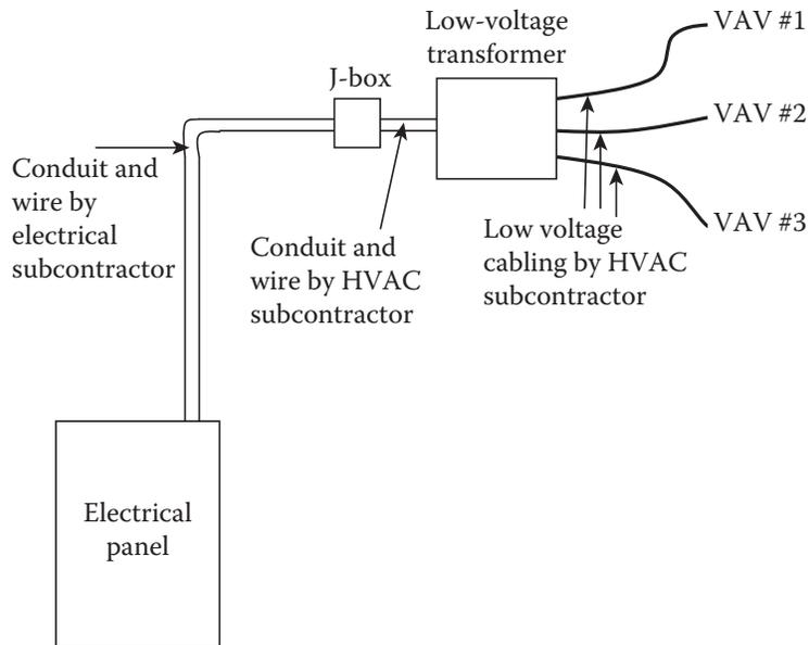
**FIGURE 40.5** Power to VAVs and FSDs.
