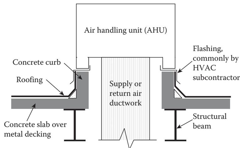
**FIGURE 40.8** Cap flashing at equipment pad.
