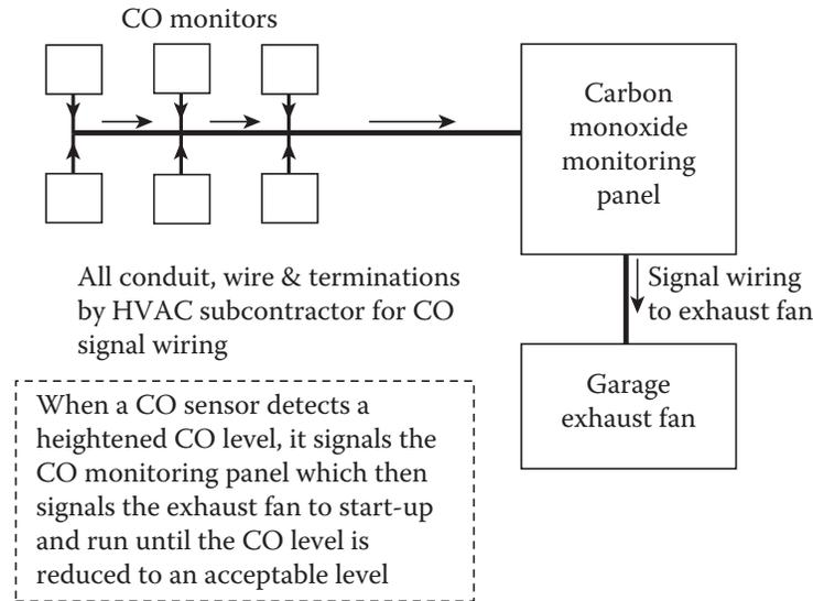
**FIGURE 40.7** Carbon monoxide detection system.
